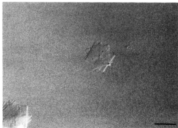
Figure 1. Transmission electron micrograph of PEO 105 crystals grown at T = 17\text{ }^{\circ}\text{C} . Bar 1\text{ }\mu\text{m} .
